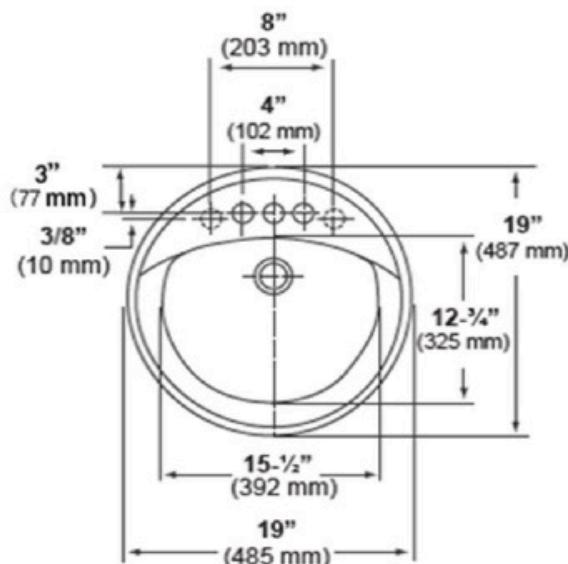
Dimensions may vary (+) or (-) 1/4". Dimensions shown in parentheses are in millimeters: 25.4 mm = 1 inch. Note: Fixture dimensions are nominal and conform with dimension and performance requirements of ASME A112.19.2-2008/CSA B45.1-08 standards. PSI rating: 20 minimum to 80 maximum per ASME A112.19.2-2008/CSA B45.1-08 standards. Dimensions subject to change or cancellation without notice. Briggs is not responsible for the use of superceded or voided specification information.
