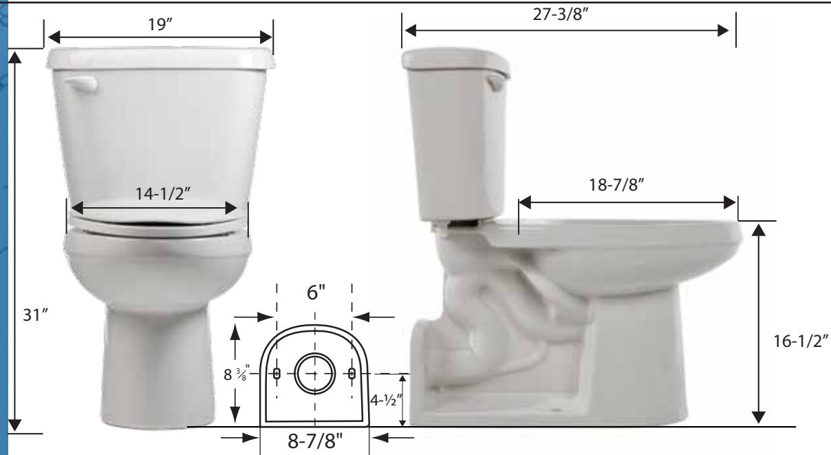
Dimensions may vary (+) or (-) 1/4". Dimensions shown in parentheses are in millimeters: 25.4 mm = 1 inch. Note: Fixture dimensions are nominal and conform with dimension and performance requirements of ASME A112.19.2-2008 / CSA B45.1-08 standards. PSI rating: 20 minimum to 80 maximum per ASME A112.19.2008 / CSA B45.1-08. Dimensions subject to change or cancellation without notice. Briggs is not responsible for the use of superceded or voided specification information.
